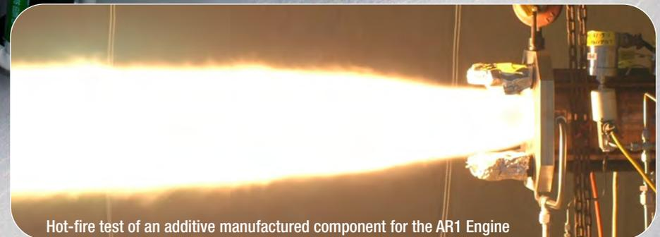
Hot-fire test of an additive manufactured component for the AR1 Engine
